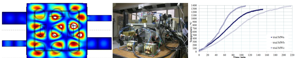
Figure 1 – Microwave furnace, electromagnetic field simulation and temperature sintering curves.
