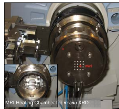
Micro-Diffraction PreFIX & Monocapillary
