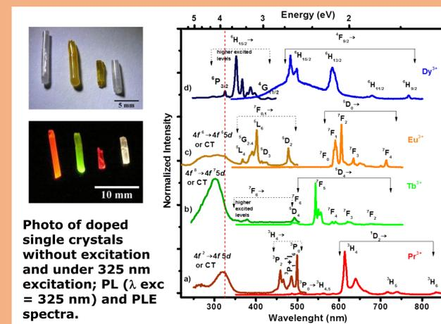
Photo of doped single crystals without excitation and under 325 nm excitation; PL ( $\lambda_{exc} = 325$  nm) and PLE spectra.
