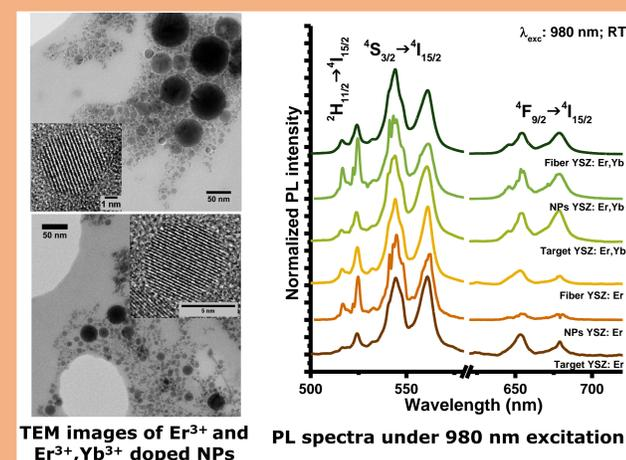
TEM images of Er<sup>3+</sup> and Er<sup>3+</sup>, Yb<sup>3+</sup> doped NPs PL spectra under 980 nm excitation
