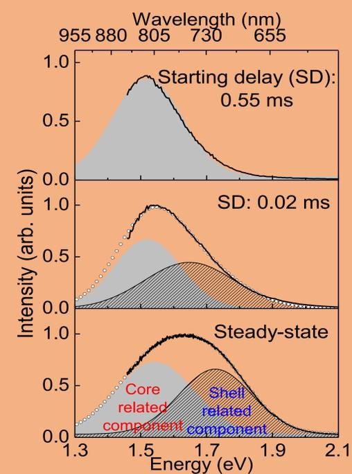
**FIG. 2** – Low-temperature (12 K) time-resolved emission spectra of surface oxidized SiNPs excited at 365 nm at SD values of 0.55 and 0.02 ms, together with steady-state emission spectrum excited at 275 nm.
