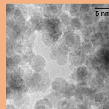
**FIG. 1** – Transmission electron microscopy of hydrogen terminated SiNPs, produced by plasma-assisted decomposition of silane.
