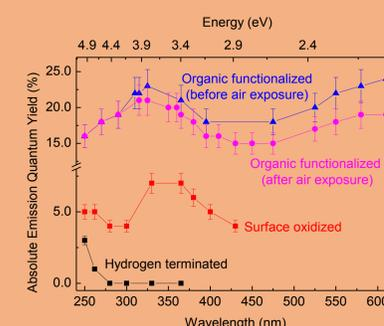
**FIG. 3** – Absolute emission quantum yield values as function of the excitation wavelength for SiNPs with different surface terminations (processed as a film).
