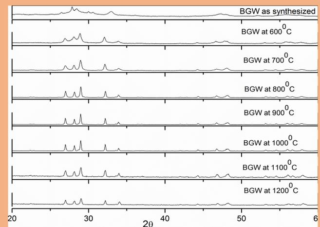
XRD patterns of BGW prepared by sol-gel method with different calcination temperatures
