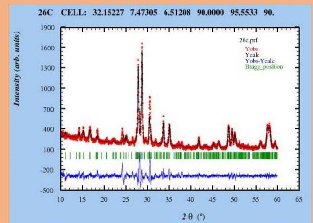
XRD patterns of BGW prepared by solid state reaction
