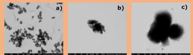
STEM micrographs of a) as-received, b) functionalized via 1,3 dipolar cycloaddition and c) functionalized xGnP followed by grafting with maleic anhydride.
