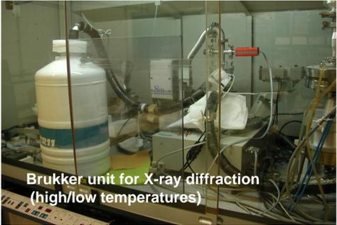
Bruker unit for X-ray diffraction (high/low temperatures)
