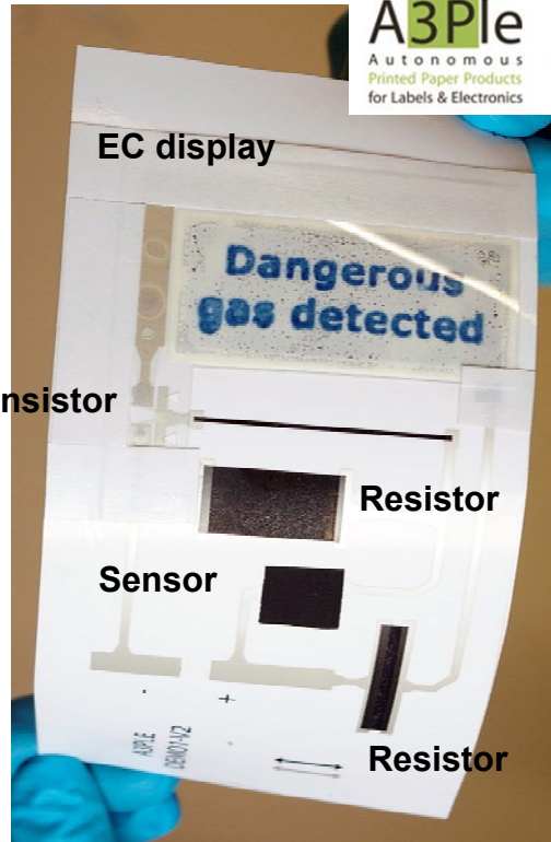
Inkjet/screen printed, all-solid-state, bendable, paper display Printed circuits and transistors.
