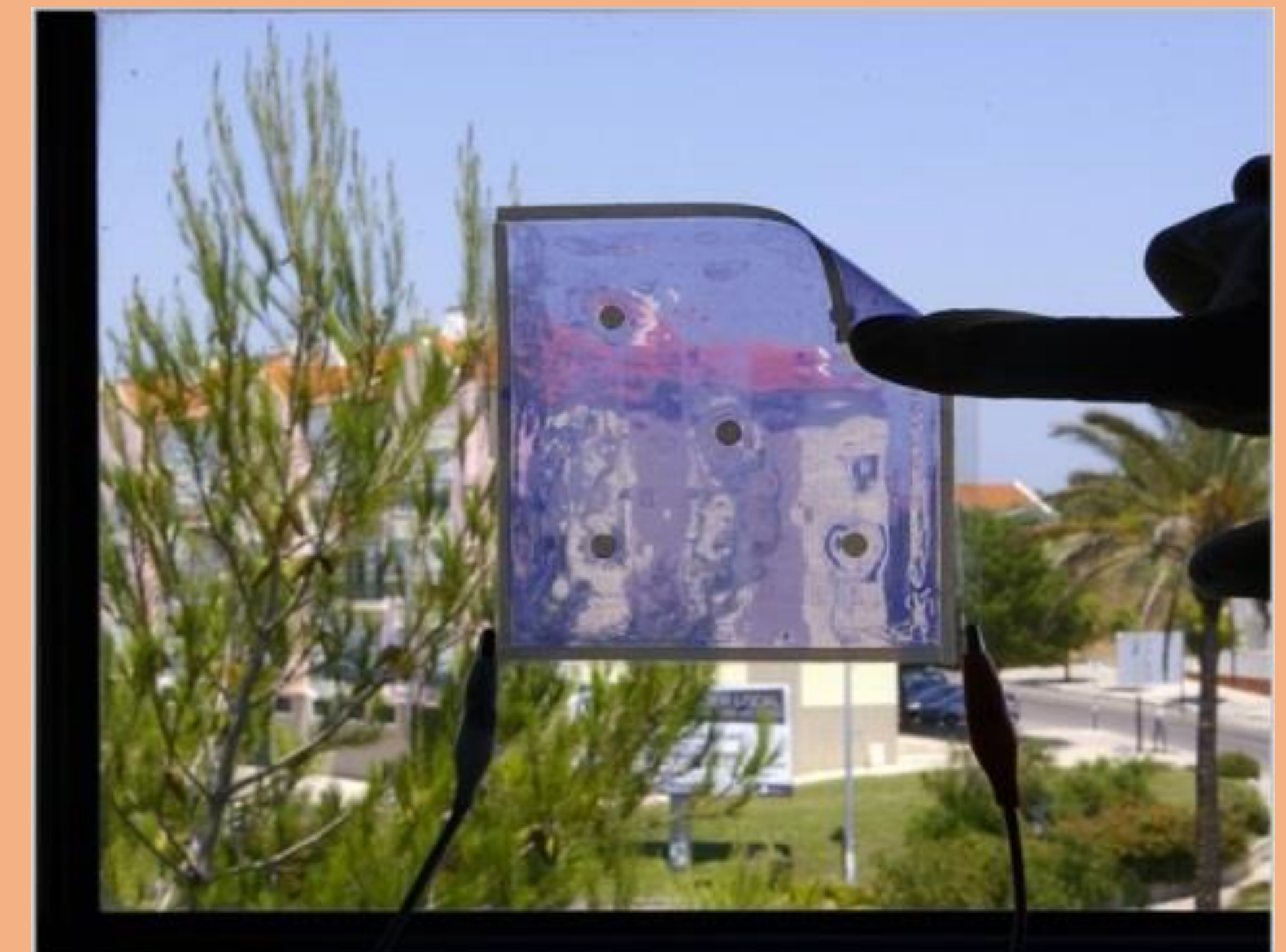
Inkjet printed, all-solid-state, beddable, large area EC window
