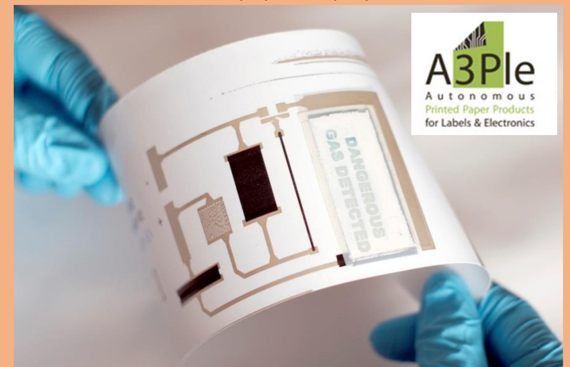
Paper EC display integrated with printed backplane
